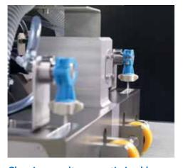
Cleaning results are optimised by the finely tuned interaction between the cleaning chemical, the water, and the brushes rotating in different directions.
