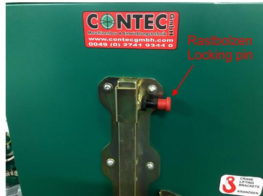
Pull the locking pin and turn it 90°. Attention: When you pull the second locking pin the unit can fall down. This can be prevented by holding the lifting arm in its position and then moving it up. Turn the locking pins again 90° and lock them in the lower position.
