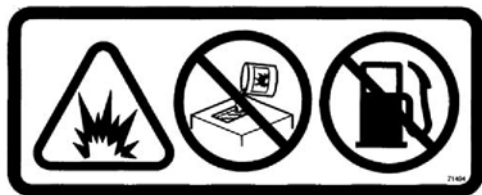
FLAMMABLE MATERIALS LABEL - LOCATED UNDER THE SOLUTION FILL PORT AND NEXT TO FOOT PEDALS
