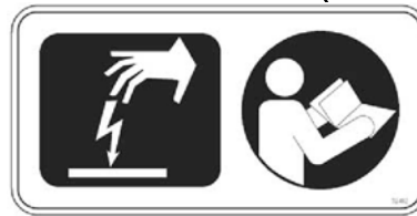
ELECTRICAL COMPONENTS, USE GROUNDING STRAP BEFORE OPENING PANEL LABEL - LOCATED ON ELECTRICAL PANEL UNDER THE SEAT
