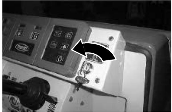
**Start:** Turn the key all the way clockwise. Release the key as soon as the engine starts.
