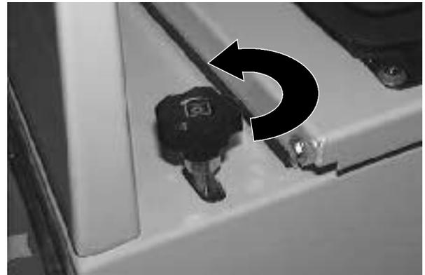
To decrease the width of the main brush pattern, turn the main brush down pressure knob clockwise.
