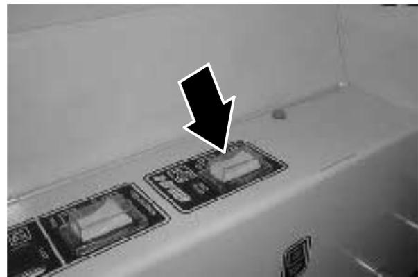
Main Brush Down and II Speed: Press the rear **II Speed**™ position of the switch.
