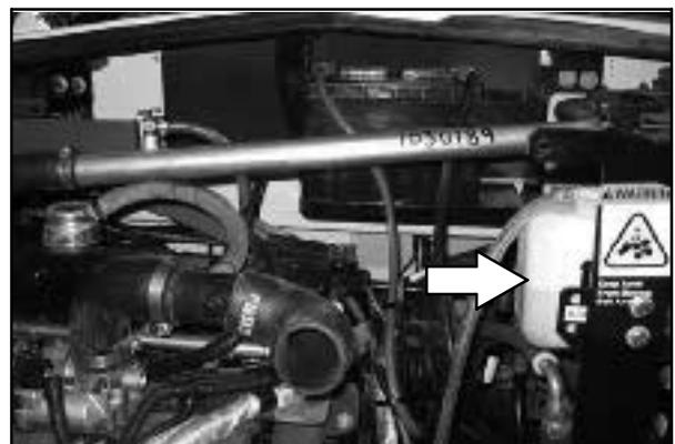
Check the radiator hoses and clamps every 200 hours of operation. Tighten the clamps if they are loose. Replace clamps if they no longer tighten properly. Replace hoses if they become hard, cracked, or swollen.
