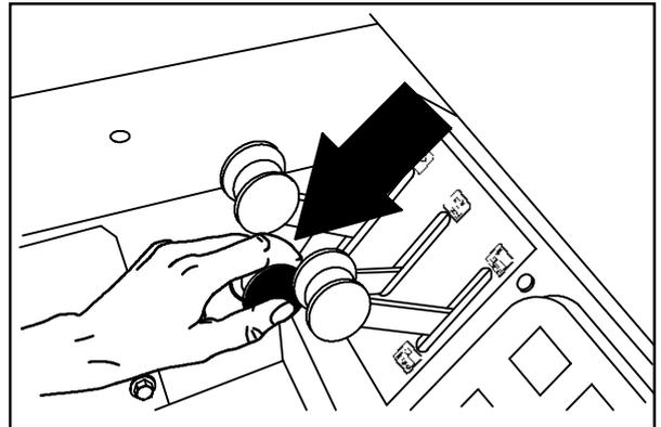
Hold: Release the hopper rollout lever into the middle position.
