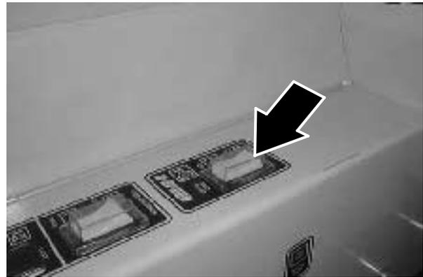
Main Brush Up and Off: Place the switch in the middle **Off** position.
