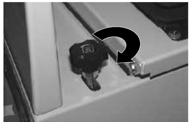
If the main brush pattern is tapered, more than 15 mm (0.5 in) on one end than the other, adjust the taper at the drive end of the brush.
