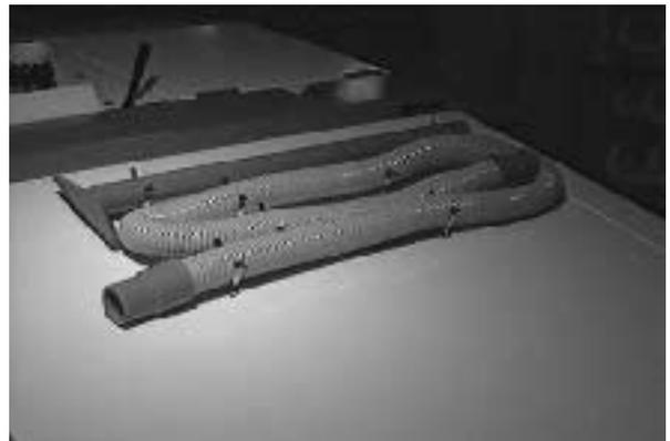
16. Replace the vacuum plug into the vacuum adaptor tube in front of the hopper, disengage the lift arm and close the forward hopper access door.
