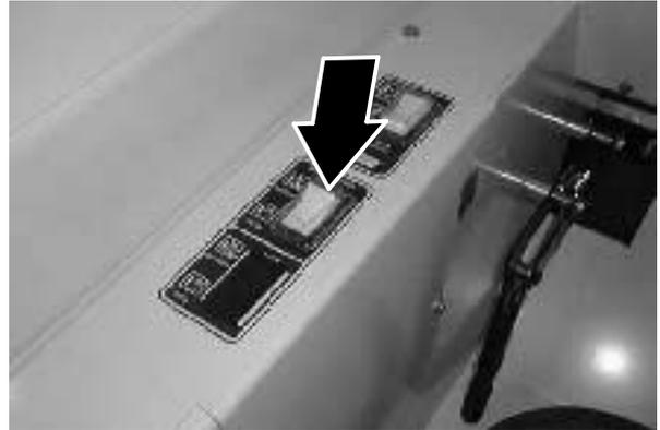
6. Press the vacuum fan switch to start the vacuum.
