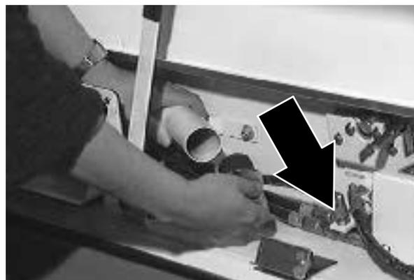
7. Remove the vacuum wand and hose from the mounting clips and assemble them together.
