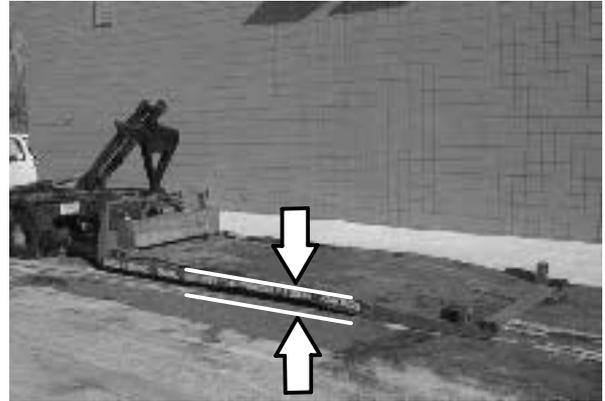
3. To winch the machine onto the truck or trailer, attach the winching chains to the rear tie down locations.
