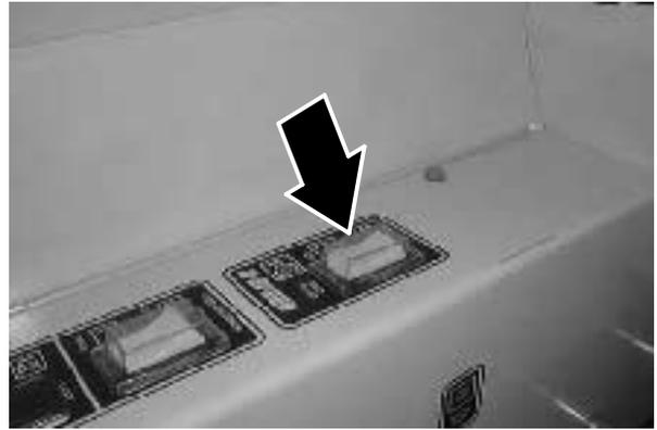
5. Push the top of the side brush switch into the **On/Down** position.
