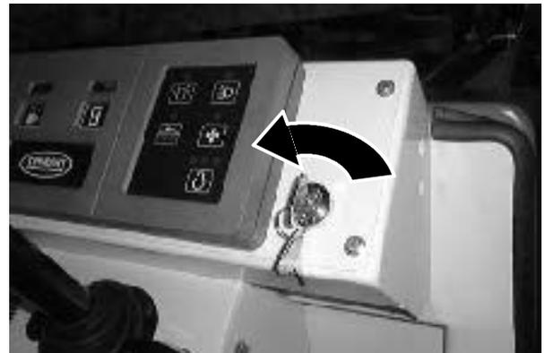
**DISENGAGING HOPPER SUPPORT BAR**
