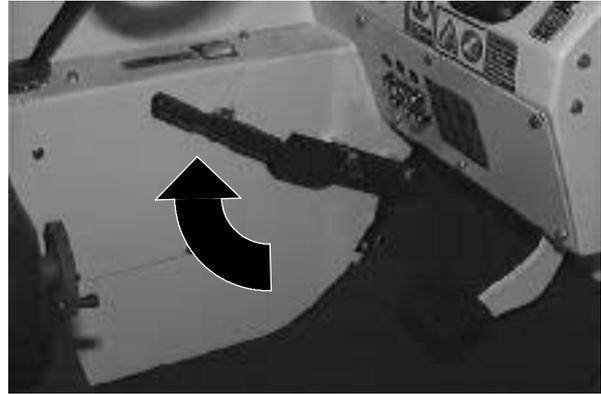
6. Turn the ignition switch key counter-clockwise to stop the engine. Remove the switch key.
