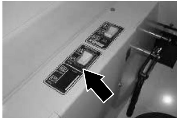
5. Open the forward hopper access door and engage the lift arm.
