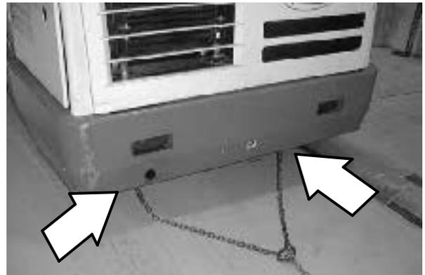
The rear tie-down locations are through the U-bolt section of the main frame under the side bumpers toward the rear.
