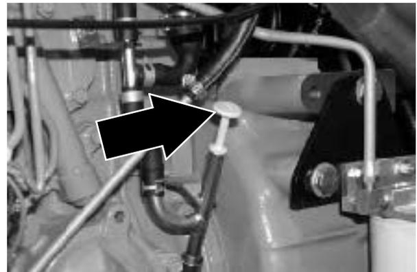
The engine oil drain is located on the engine oil pan. Drain the engine oil when it is warm.
