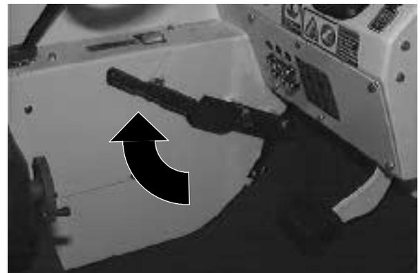
Release: Push the parking brake lever down.
