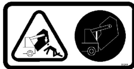
HOPPER SUPPORT LABEL - LOCATED ON LEFT HOPPER LIFT ARM AND BOTH SIDES OF THE HOPPER COMPARTMENT.
