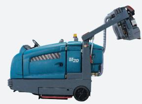
Cleaning productivity is increased with a large 110 liter, 177 kg debris hopper with 152 cm variable dump height.
