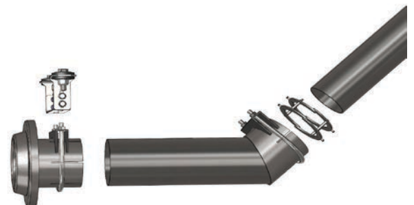
Image: possible tailpipe configuration
