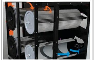
The effective RamAir™ pulse amplifier: individually cleaning of the filter cartridges by compressed air pulses.
