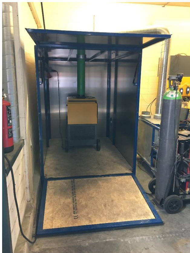
Figure 3-4 MobileGo placed in the test cabin with the upstream duct connected to the inlet
