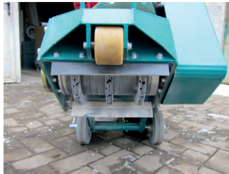
variable diamond drum - max. cutting depth 10 mm
