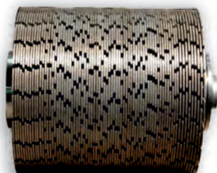
variable diamond drum - max. cutting depth 10 mm
